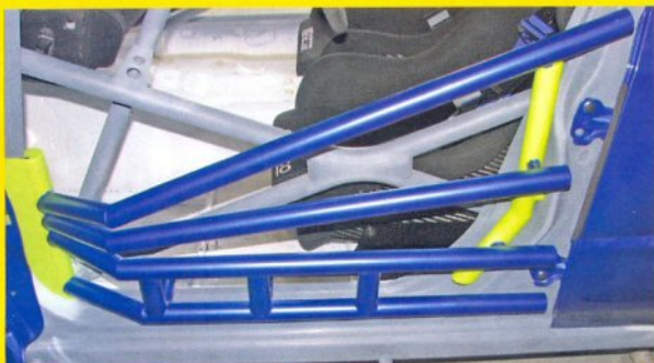
Load-spreading door bars, inspired by those used in NASCAR, were developed by the FIA Institute in 2005
