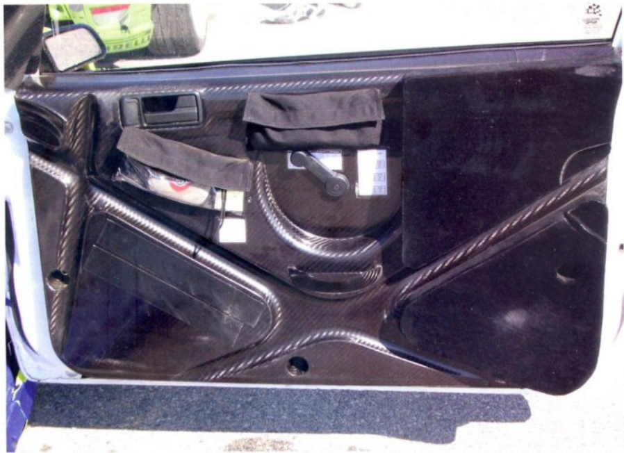
An alternative solution to side impact protection is this carbon fibre cover over a foam structure. Note the troublesome factory window winder still in situ
